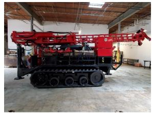
DC Water's contractor will use a drill rig (pictured) that is approximately 7 feet wide, 15 feet long, and 10 feet tall during the process. Support vehicles (pick-up trucks) will also deliver staff and supplies to each boring site. Borings will be finished at the surface with a flush-mount well cover. Before the team demobilizes from the site, they will clean the work area, remove all drilling equipment and debris, and restore the pavement or grass.
