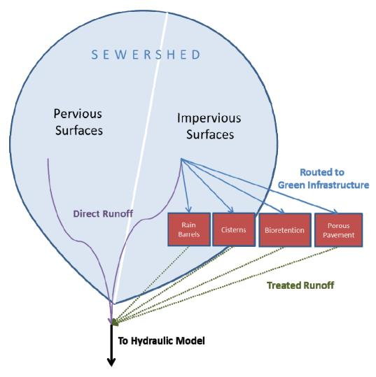
Figure 4-3: SWMM5 LID control routing
