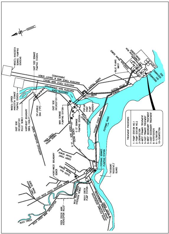
Figure 2-1. Combined Sewer System Schematic
