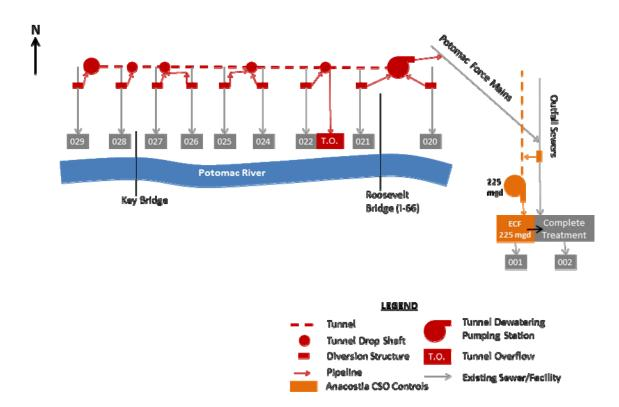
Figure 5-5. LTCP Potomac Tunnel Schematic
