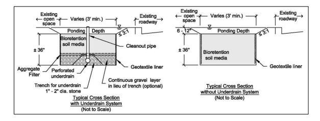
Figure 5-4. Schematic of typical vegetated swale with and without underdrain system. (Source: Wetland Studies and Solutions, Inc.)
