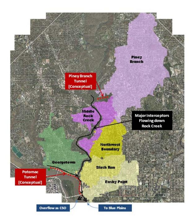
Figure 5-2. Drainage Areas Serving Potomac and Piney Branch Storage Tunnels
