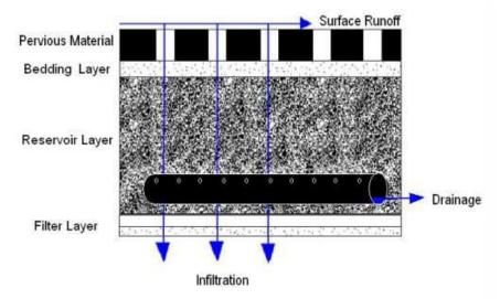
Figure 3-4. Typical cross-section of pervious pavement. (Source: VA SWM BMP Design Specifications)
