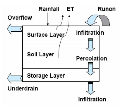
Figure 3-2. Conceptual Model of LID Bioretention Cell in SWMM5
