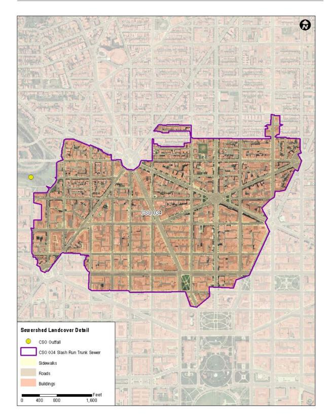
Figure A-11. Sewershed Characteristics - CSO 034, Slash Run Trunk Sewer
