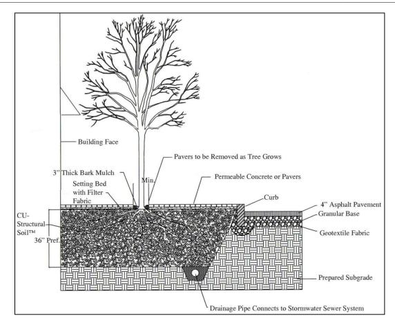
Figure 4-4. Typical CU-Structural Soil<sup>™</sup> application incorporating pervious pavement. (Source: Cornell University – Urban Horticulture Institute)
