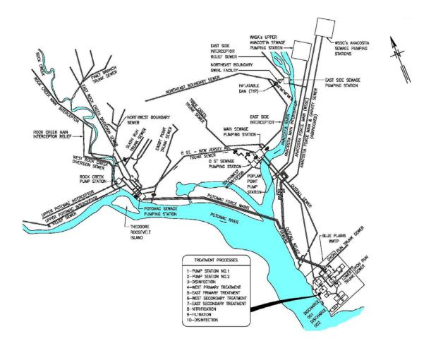
Figure 5-1. Sewer System Schematic
