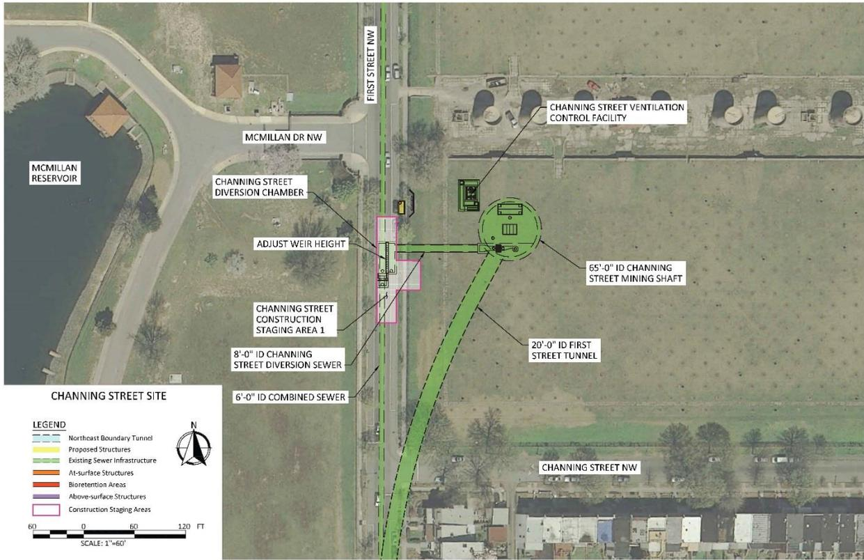
Figure 3-7: Channing Street Mining Shaft Site
