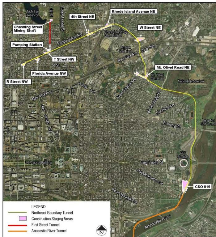
Figure 2-1. NEBT Alignment and Construction Sites
