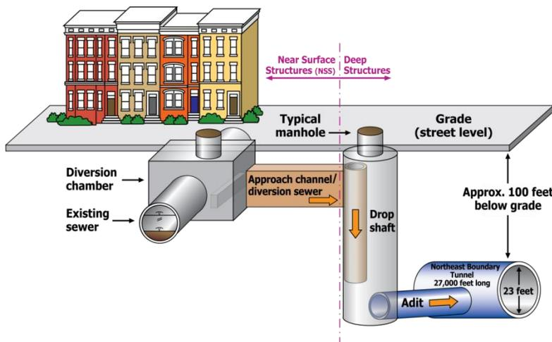
Figure 2-2: Graphic illustration of a typical diversion facility
