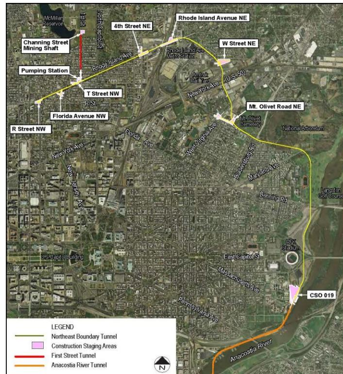
**Figure 2-1. NEBT Alignment and Construction Sites**
