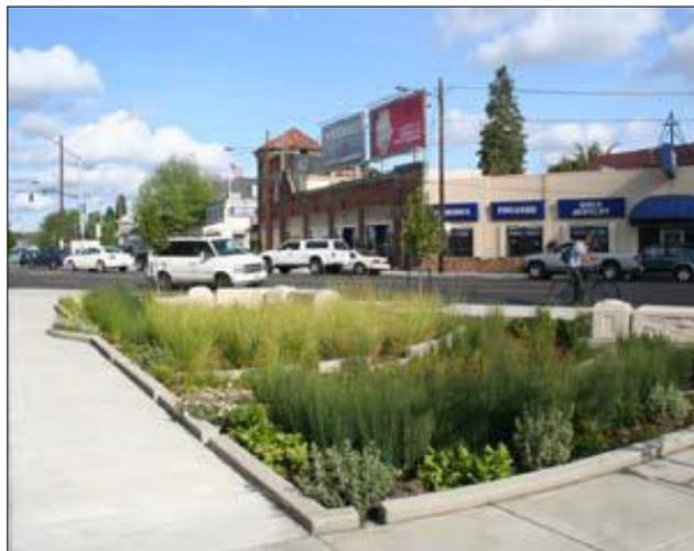
**Figure 2-2. Small bioretention facility retrofitted in a busy urban setting.
