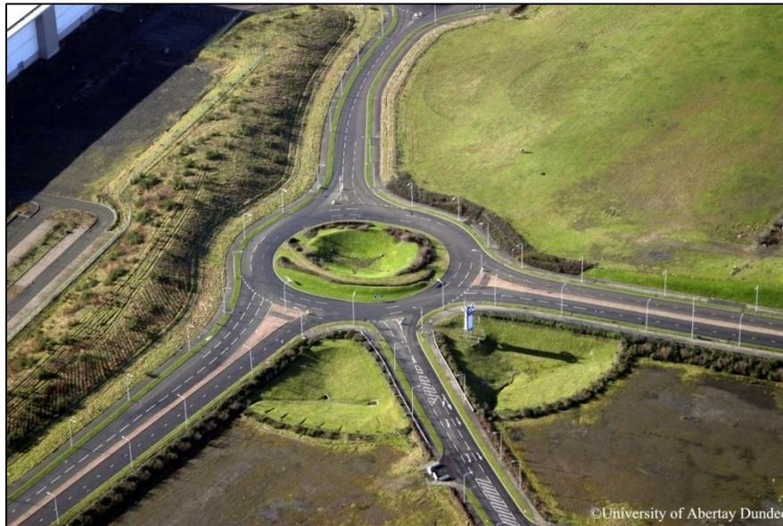
**Figure 3-18. Green detention basin at DEX roundabout.
