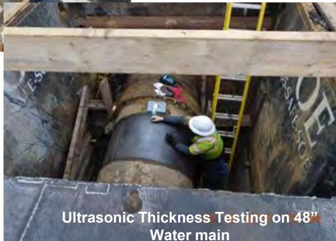
Ultrasonic Thickness Testing on 48" Water main
