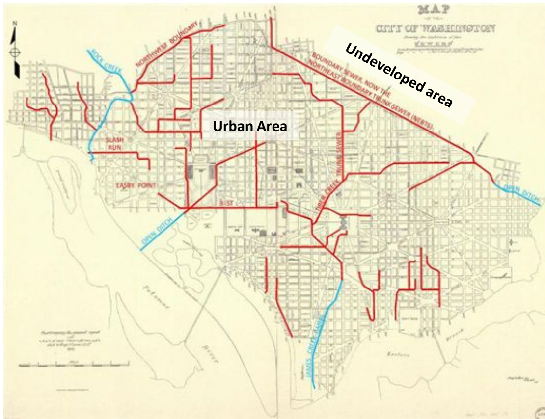
— Principal Sewers With Discharge to Potomac and Anacostia Rivers and Rock Creek
