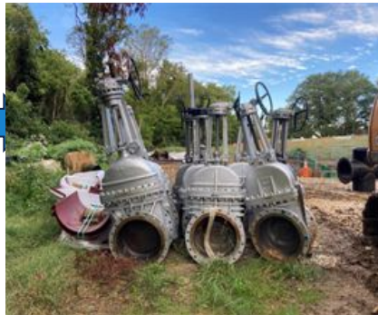
Bypass Pipe Valves
