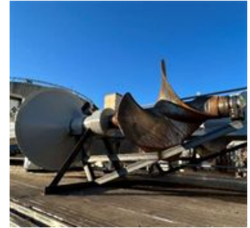
Refurbished mixer propellers
