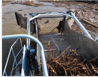
debris a month. Skimmer boats have efficiently removed as much as 120 tons of trash in one month during rainy weather. By removing such waste and pollutants, our rivers are cleaner and safer for everyone, including their natural inhabitants.
