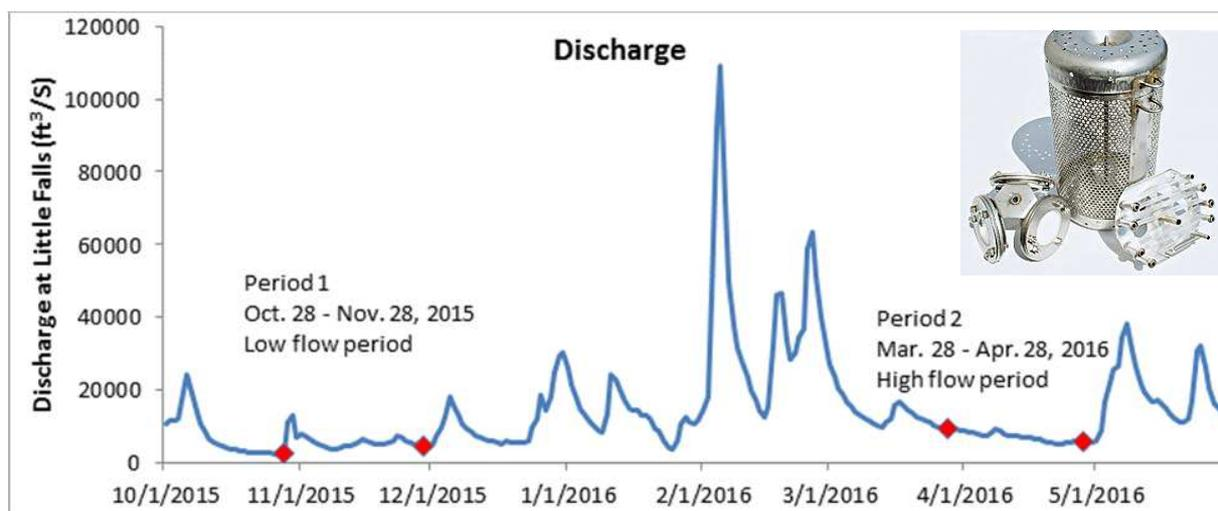
Figure 5. Discharge at Little Falls, Potomac River, and highlighting periods of POCIS Deployment. Inset image of POCIS Samplers.
