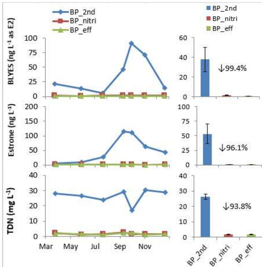
Figure 6: Seasonal variability and mean values for estrogenic activity, estrone, and nitrogen treatment profiles at Blue Plains. Note: BP = Blue Plains, 2<sup>nd</sup> = Post Secondary treatment, nitri = post advanced nutrient control, eff = plant effluent.
