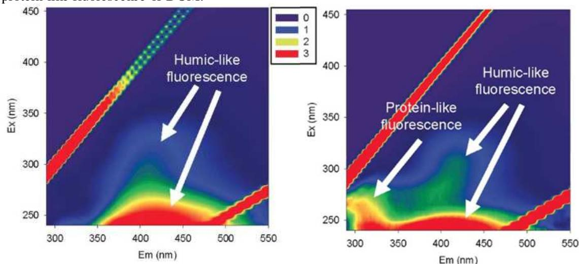
Figure 14: Example EEMs. Taken from Fu et al (2015)
