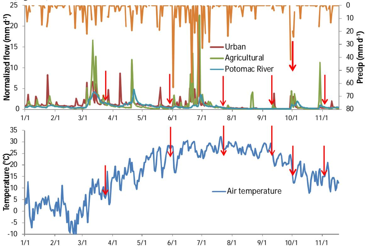
**Figure 4 Daily precipitation, air temperature (at DC Reagan International Airport), and runoff from Potomac River watershed (estimated from flow at Little Falls). Red Arrows Represent Sampling events, providing precipitation and temperature data for the surrounding period.**
