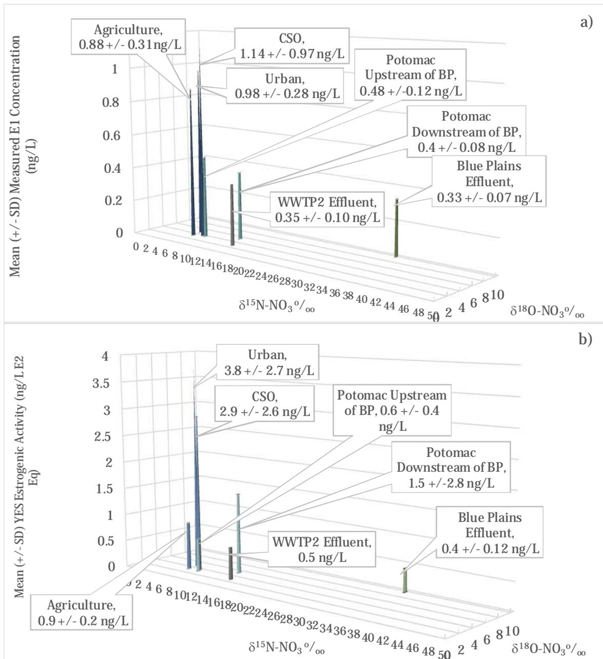
Figure 17: Comparing Nutrient Fingerprints with EDCs (a) estrone, and b) BLYES activity)
