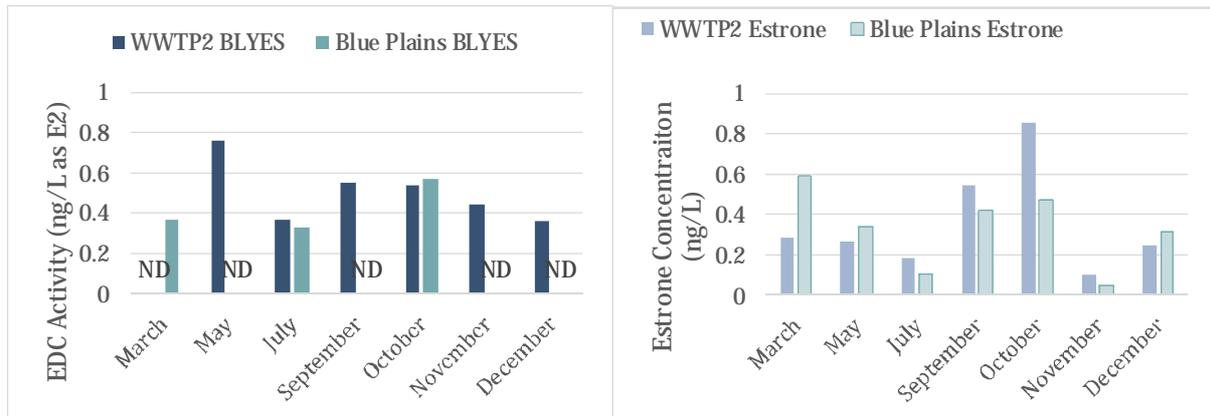
**Figure 11: Effluent Concentrations of EDCs from Blue Plains and WWTP2. Both facilities employ advanced nutrient control technologies.**
