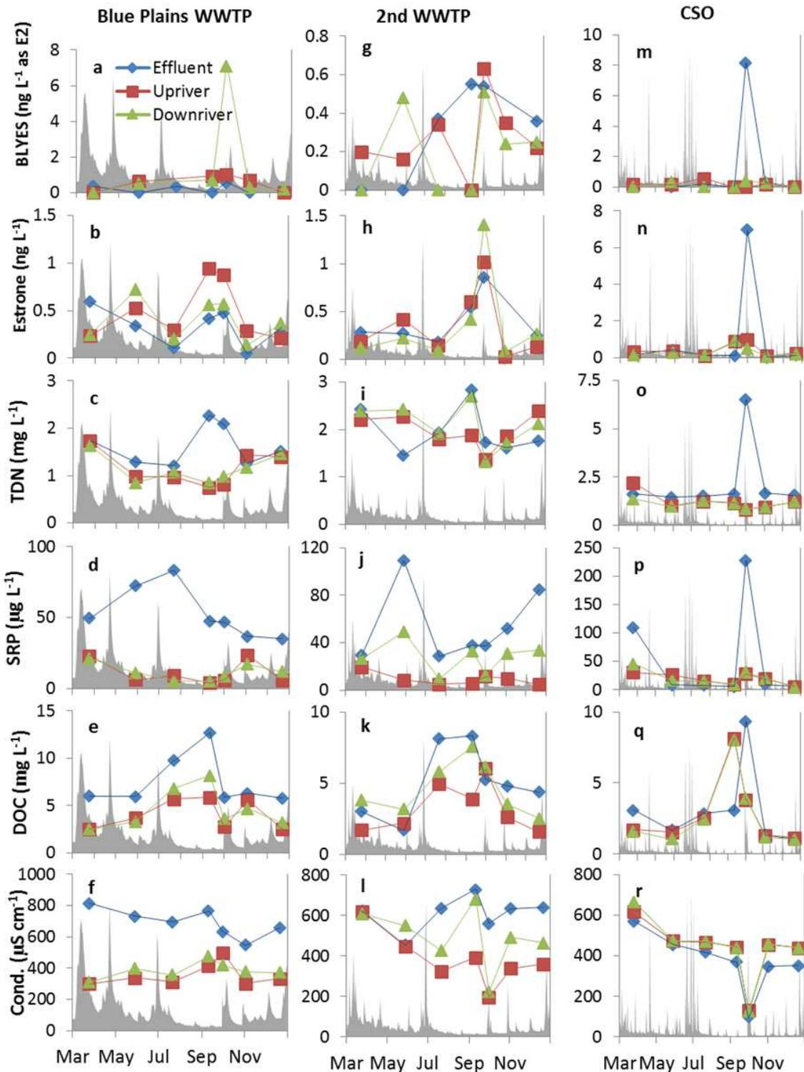
Figure 9: Concentrations of estrone, TDN, SRP and DOC of upriver, downriver, and in the WWTP or CSO effluent. Potomac hydrograph shown in the background.
