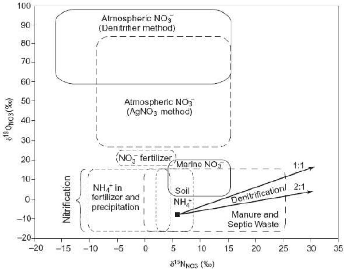
**Figure 13. Typical values of N and O isotope ratios (expressed in  $\delta^{15}\text{N-NO}_3$  and  $\delta^{18}\text{O-NO}_3$  values) of nitrate derived from various N sources. Taken from Kendall et al, 2007.**
