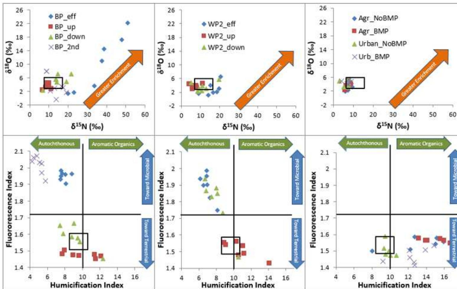
Figure 9: Nutrient and NOM fingerprinting techniques for Blue Plains, WWTP2, and the non-point sources to the Potomac. The black box on each plot summarizes ranges of eEDCs considered as “background” in the Potomac. BP = Blue Plains WWTP, WP 2 = Second tested WWTP, Agr = Agricultural Site, Urb = Urban Site. Eff = effluent, up = Upstream, down = Downstream, BMP = Best Management Practices, No BMP = Lacking Best Management Practices.
