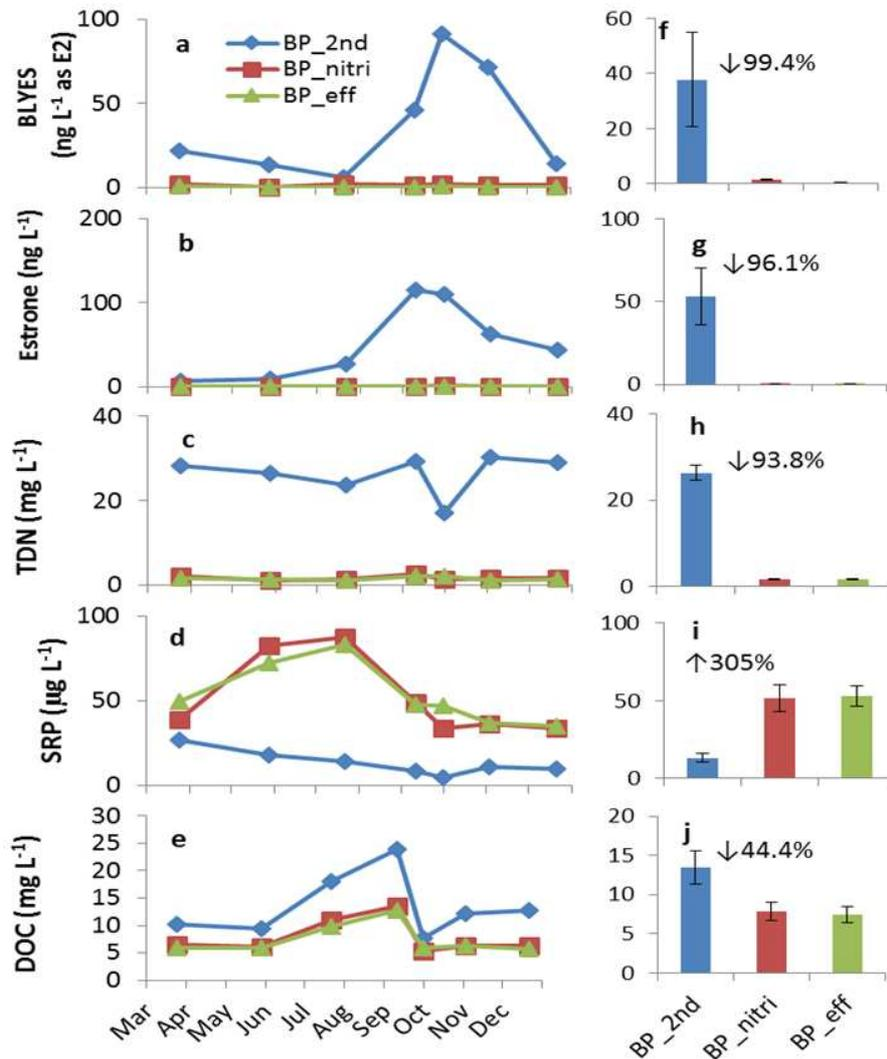
**Figure 10: Seasonal and mean values of estrogenic activity, estrone, TDN, SRP and DOC, measured as a profile from Blue Plains (BP) post-second treatment (BP\_2<sup>nd</sup>) to post-nitrification/denitrification (BP\_nitri) to outfall (BP\_eff).**
