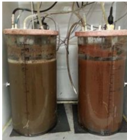
Exhibit A. Bench Scale SBR Setup.
