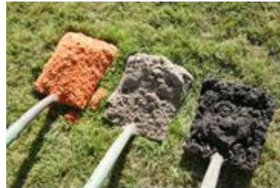
TAGRO Mix components: sawdust, sand and Class A biosolids
