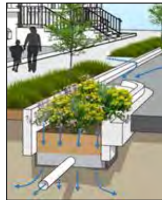
Curb Extension Bioretention
