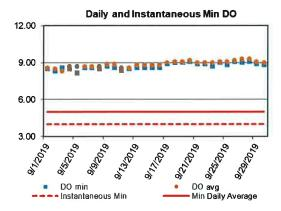
Dissolved Oxygen (DO) is a measure of the atmospheric oxygen dissolved in water. The DO readings for the month are within the permit limits. The minimum daily average is 8.3 mg/L. The minimum instantaneous DO reading is 8.2 mg/L. The minimum daily average and instantaneous permit limits are 5.0 mg/L and 4.0 mg/L, respectively.
