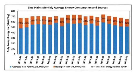
The graph above is based on power monitors installed at the Main Substation and CHP, and reflects average energy consumed at Blue Plains in MWH/day. Of the total use, the energy purchased from PEPCO and net energy supplied by CHP are indicated by the blue and orange highlights, respectively.
