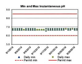
pH is a measurement of acidity of the effluent. The minimum and maximum pH observed were 6.6 and 6.8 standard units, respectively. The pH was within the permit limits of 6.0 and 8.5 for minimum and maximum respectively.
