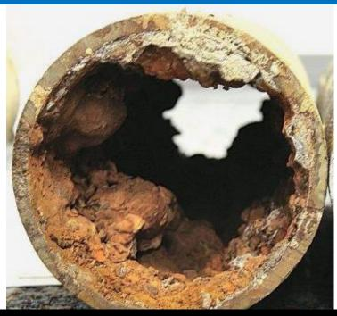
Small Diameter Water Main unlined Cast Iron pipe
