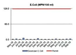
E. coli is an indicator of disease causing organisms (pathogens). The E. coli permit limit is 126/100mL. The E coli geometric mean is 2.9 /100mL, and well below the permit limit.
