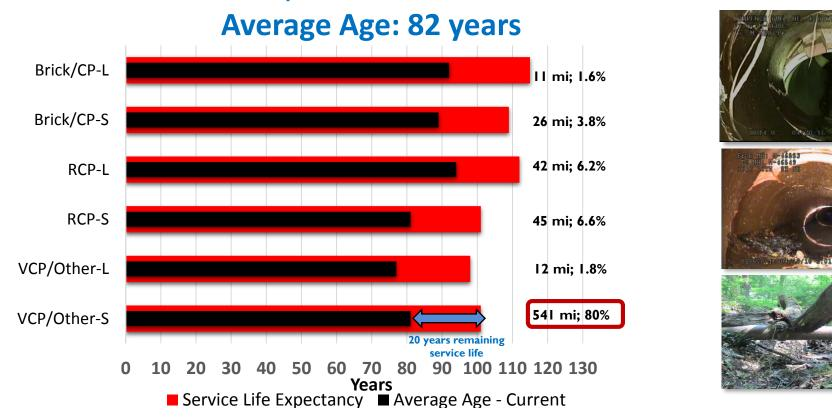
Note: CP=Concrete Pipe; RCP=Reinforced Concrete Pipe; VCP=Vitrified Clay Pipe; L=Large; S=Small
