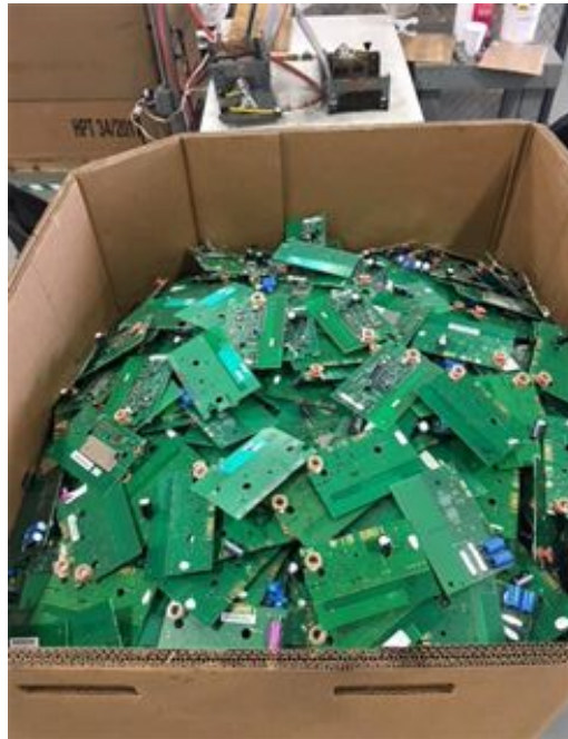
Gaylord storage with fully disassembled PCBs
