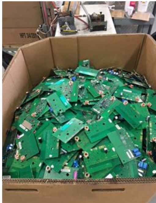
Gaylord storage with fully disassembled PCBs
