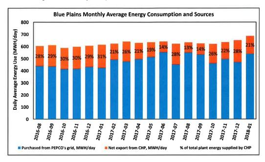
The graph above is based on power monitors installed at the Main Substation and CHP, and reflects average energy consumed at Blue Plains in MWH/day. Of the total use, the energy purchased from PEPCO and net energy supplied by CHP are indicated by the blue and orange highlights, respectively.
