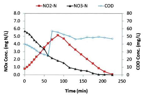
**Figure 2**. Batch bioassay test with nitrate [NO3-N] and acetate [COD] added under anaerobic conditions. Nitrite increases during the first half of the test indicating partial denitrification [NO3-N → NO2-N] is occurring.
