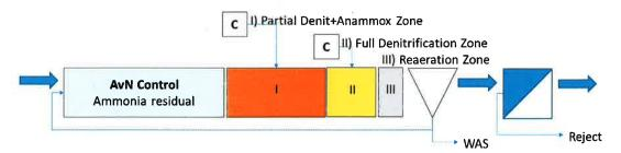
**Figure 1.** Shortcut nitrogen removal process with integrated post-polishing zones. Treatment phases include an aeration stage using AvN control followed by 3 post polishing cells. A similar concept could potentially be applied at Blue Plains AWTP in the existing nitrogen removal process.
