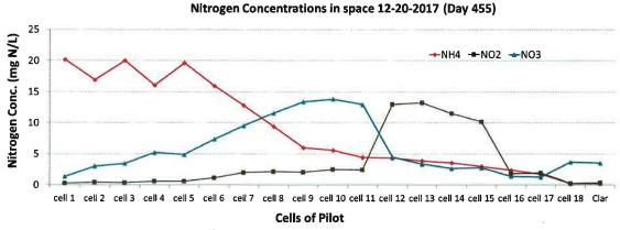
**Figure 3**. Nitrogen species concentration profile along the pilot process. Cells 1 through 10 are aerated and air is controlled using the AvN strategy, while Cells 11 through 17 are mixed [no aeration]. Acetate is dosed in cells 12, 14 and 16. Cell18 is aerated to mimic the full scale plant's operation for reaeration. Profile shows total nitrogen less than 5 mg N/L was achieved.
