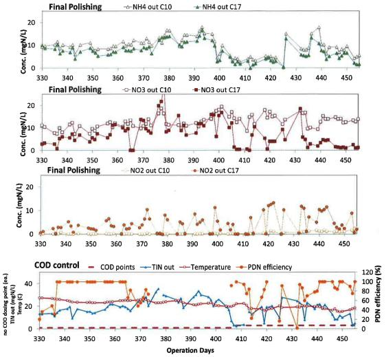
**Figure 4**. The shortcut nitrogen removal pilot data for Cells 10 and 17. Cell 10 is the last cell before the polishing zone which is comprised of Cells 11 through 17. Cell17 is the last cell in nitrogen polishing before reaeration and is representative of the post-polishing zone effluent.
