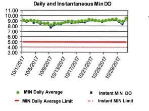
Dissolved Oxygen (DO) is a measure of the atmospheric oxygen dissolved in wastewater. The DO readings for the month are within the permit limits. The minimum daily average is 8.2 mg/L. The minimum instantaneous DO reading is 7.7 mg/L. The minimum permit limits are 5.0 mg/L and 4.0 mg/L respectively.
