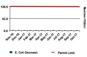
E.coli is an indicator of disease causing organisms (pathogens). The E.coli permit limit is 126/100mL. The E coli geometric mean is 1.0 /100mL, and well below the permit limit.
