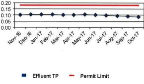
The Total Phosphorus (TP) is a measure of the particulate and dissolved phosphorus in the effluent. The annual average effluent TP = concentration is 0.10 mg/L, which is below the 0.18 mg/L annual average limit.
