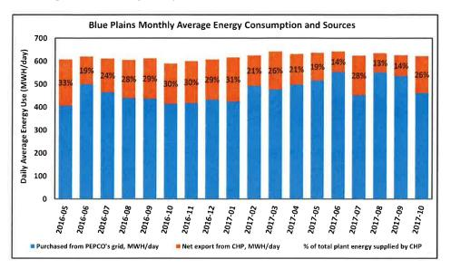
The graph above is based on power monitors installed at the Main Substation and CHP, and reflects average energy consumed at Blue Plains in MWH/day. Of the total use, the energy purchased from PEPCO and net energy supplied by CHP are indicated by the blue and orange highlights, respectively. The graph below shows the monthly value of the net electricity produced by CHP by assuming unit price of \$78/MWH of electricity.
