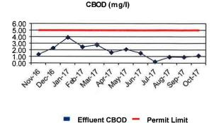
Carbonaceous Biochemical Oxygen Demand (CBOD) is a measure of the amount of dissolved oxygen required for the decomposition of organic materials. The effluent CBOD concentration averaged 1.09 mg/L (partial month), which is below the 5.0 mg/L limit.
