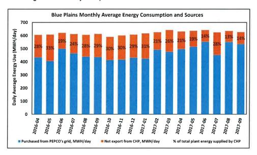
The graph above is based on power monitors installed at the Main Substation and CHP, and reflects average energy consumed at Blue Plains in MWH/day. Of the total use, the energy purchased from PEPCO and net energy supplied by CHP are indicated by the blue and orange highlights, respectively. The graph below shows the monthly value of the net electricity produced by CHP.
