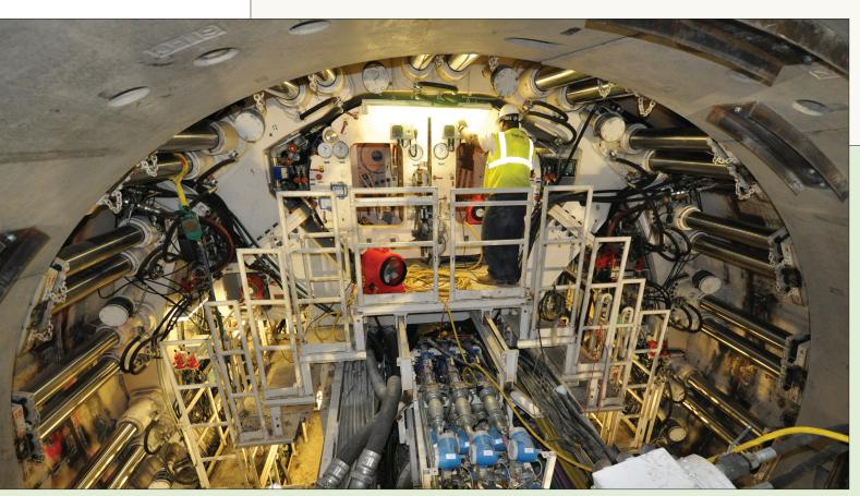
The front shield of the tunnel boring machine shows the chamber where workers must acclimate to pressure before working on the cutterhead
