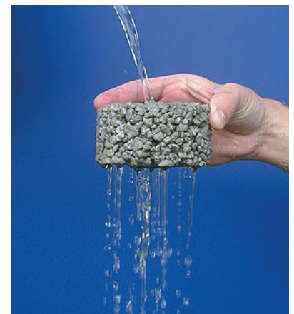
This porous pavement allows water to infiltrate the ground instead of running into the sewer system.
