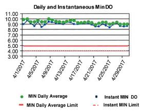
Dissolved Oxygen (DO) is a measure of the atmospheric oxygen dissolved in wastewater. The DO readings for the month are within the permit limits. The minimum daily average is 8.9 mg/L. The minimum instantaneous DO reading is 8.4 mg/L. The minimum permit limits are 5.0 mg/L and 4.0 mg/L respectively.
