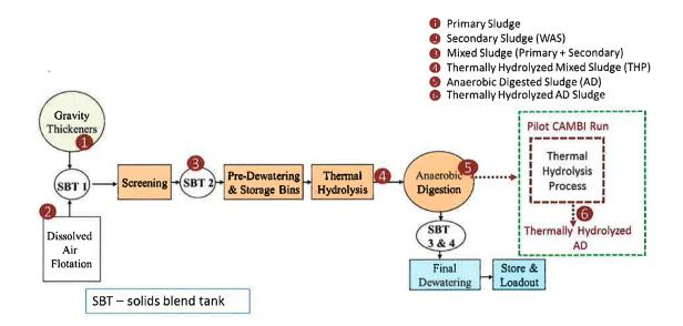
Figure 1. Schematic of Blue Plains AWTP Solids Treatment Processes and Location of Samples Collected for Dewatering Study
