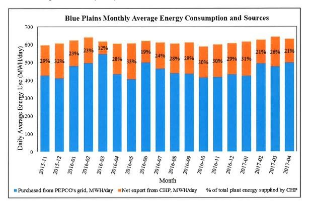
The graph above is based on power monitors installed at the Main Substation and CHP, and reflects average energy consumed at Blue Plains in MWH/day. Of the total use, the energy purchased from PEPCO and net energy supplied by CHP are indicated by the blue and orange highlights, respectively.
