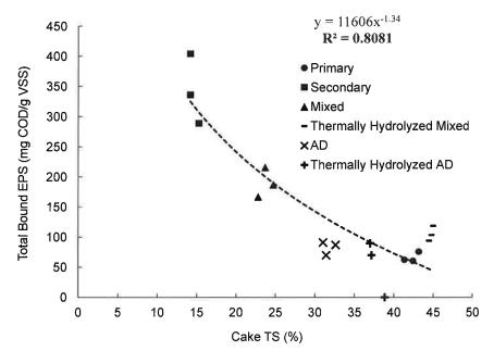
Figure 3. Global correlation between extracellular polymeric substance (EPS) and cake %TS for various sludges (Primary sludge, secondary sludge, blended/mixed sludge, thermally hydrolyzed sludge, anaerobically digested, anaerobically digested thermally hydrolyzed).
