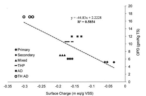
Figure 2. Global Correlation between Surface Charge and Optimum Polymer Dose (OPD) for Various Sludges (Primary, Secondary, Mixed, Thermally Hydrolyzed (THP), Anaerobically digested (AD), Thermally Hydrolyzed Anaerobically Digested (TH AD)).
