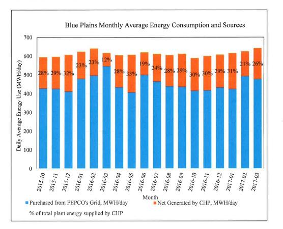
The graph above is based on power monitors installed at the Main Substation and CHP, and reflects average energy consumed at Blue Plains in MWH/day. Of the total use, the energy purchased from PEPCO and net energy supplied by CHP are indicated by the blue and orange highlights, respectively.
