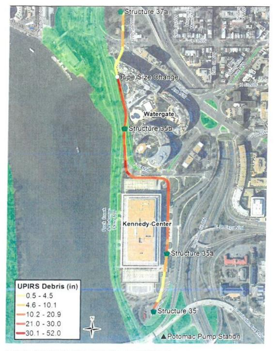
Figure 1: UPIRS Overview Map with Pre-Cleaning Debris Levels
