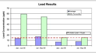
The total coliform and the lead graphs display the 2004 and 2005 water quality data and show the improvement since starting the corrosion control treatment and extensive flushing. WASA will continue researching and monitoring water quality to ensure this high water quality is maintained.
