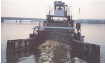
During rainy weather, the skimmer boats collect more debris than usual because of the amount of waste that is dislodged from catch basins. Since 1992. WASA has removed over 6,000 tons of trash and floatable debris from the river
