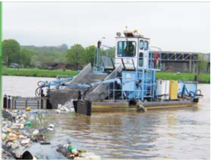
(Right) DC WASA skimmer boats work the Anacostia and Potomac rivers, capturing and removing upwards of 400 tons of trash and debris annually.
