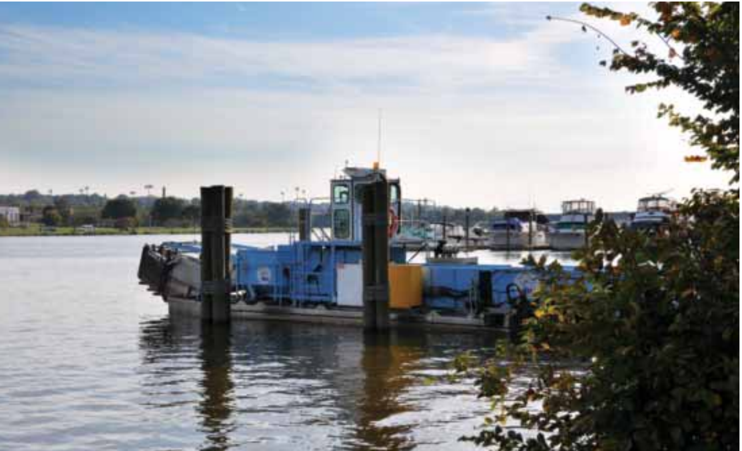
The Authority operates two skimmer boats that remove floatable debris from the Anacostia and Potomac rivers—up to 120 tons per month.
