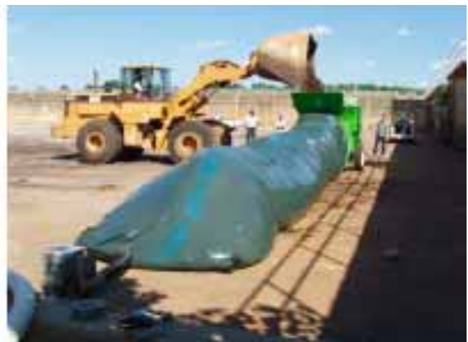
The composting system uses a silage bag as a vessel, with an aeration plenum running down the length of the bag (inside), which is attached to a blower on one end to ensure the composted material remains under aerobic conditions.
