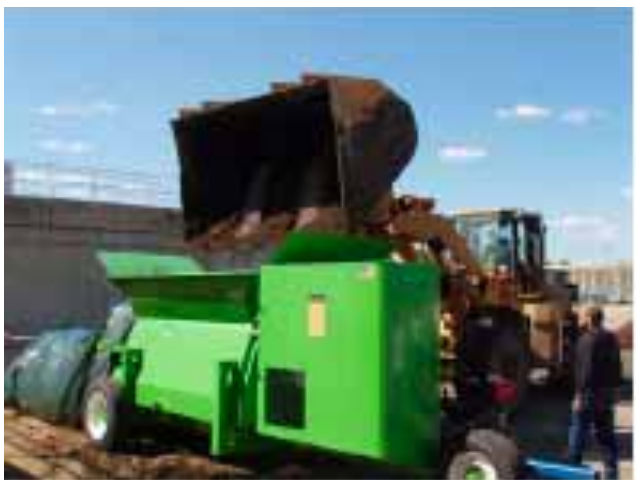
The composting system uses a silage bag as a vessel, with an aeration plenum running down the length of the bag (inside), which is attached to a blower on one end to ensure the composted material remains under aerobic conditions.
