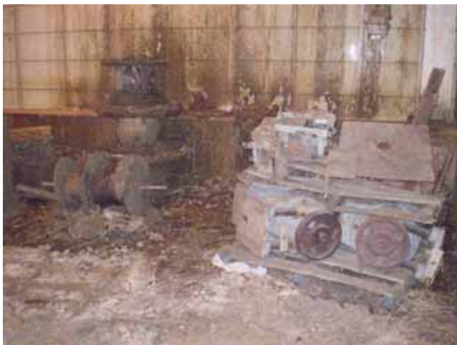
(Left): When biosolids conveyors were hosed with water, dirty water flowed through openings in the floor to lower level storage wells and areas used for equipment storage, shown here. (Right): Good housekeeping practices eliminated the need for water, and here, the equipment storage area is shown after it was cleaned up – and could remain that way.
