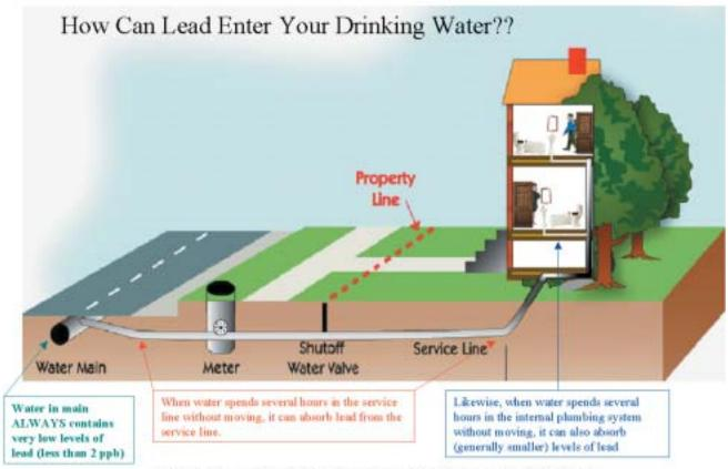
NOTE: Water moving through the service line and internal plumbing CAN pick up small amounts of lead as it flows through, but this is likely to be at a MUCH lower level.
