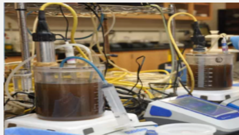
DC Water bench-scale experimental setup used to test and evaluate wastewater treatment processes
