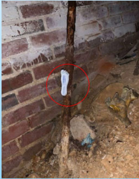
Magnet identifying galvanized pipe
