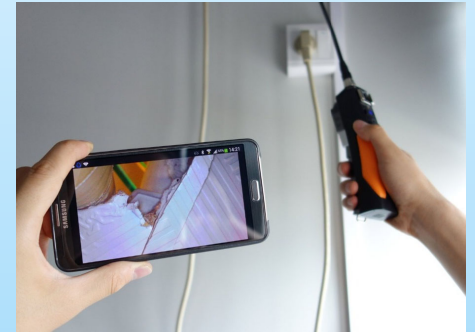
If POE not visible – consider a borescope
