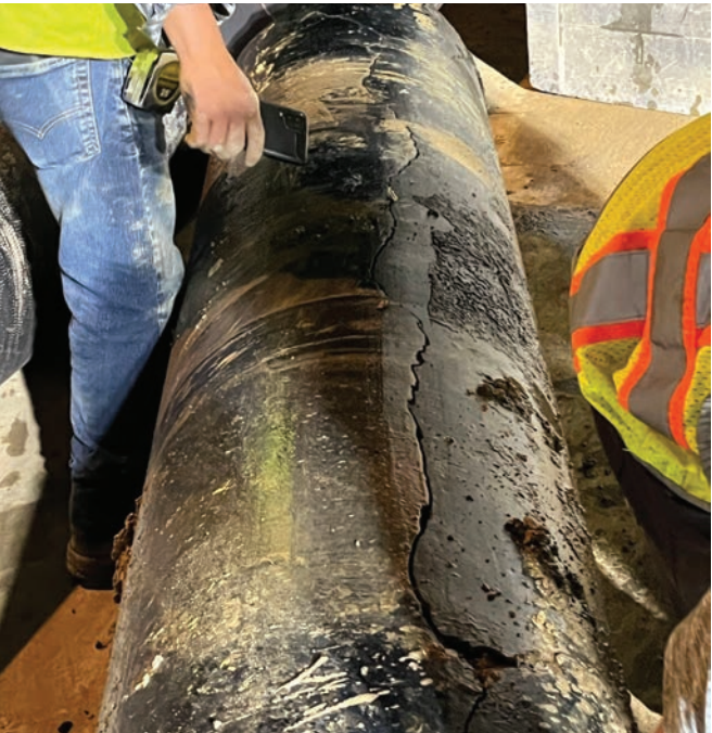
Split in a 115 year old cast iron pipe
