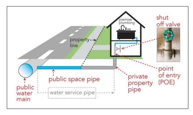
DC Water will help you identify the pipe material for your water service line. This picture shows that most of the water service line is buried and therefore not visible. However, you can look for the water pipe entry into the home to see one end of it.
