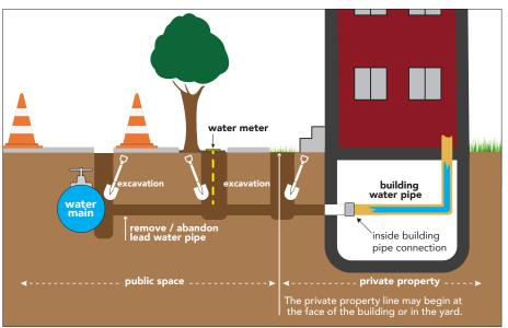
Install a new copper water pipe from the District water main in the street to your building, through the wall where the pipe comes in and connect it to the water pipe in your building.
