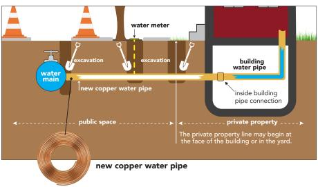
Turn on water, fill holes, restore area, and flush water from an outside hose connection, if possible.
