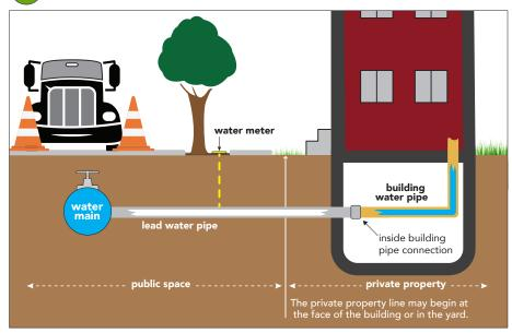
Dig down near District water main, meter and property line and remove / abandon your lead water pipe from the watermain in the street, through your building wall or floor, to the pipe connection in your building.
