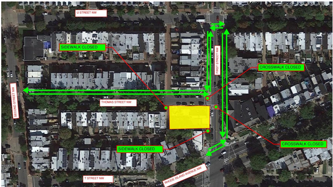
The above map shows construction sites in yellow, green arrows indicate how pedestrians will move around the construction area.
