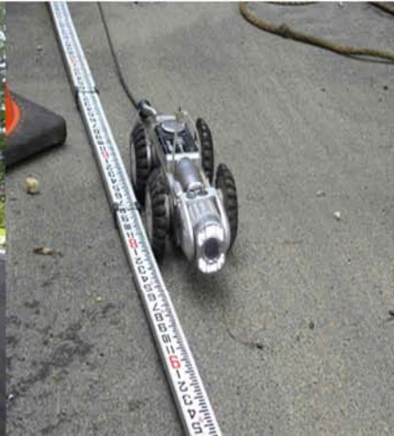
Sewer Inspection Rover
