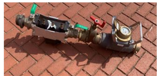
Hydrant Meter with BPA
