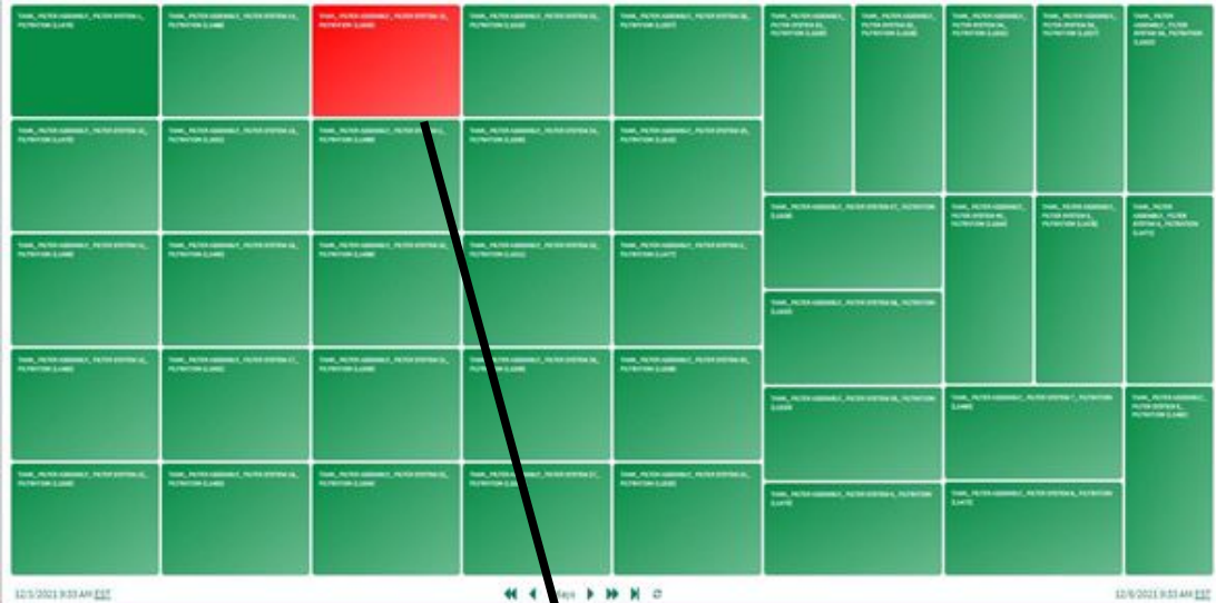
Figure 2. Interactive dashboard identifying which filters are displaying signs of failed underdrain. Each box represents the health status of one filter. There are 40 filters in total. By clicking on one of the boxes, a detailed trend is displayed for the selected filter.
