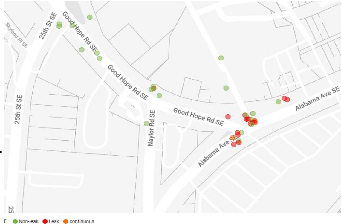
Heat map of the acoustic showing the classification of field result as non-leak, leak, is continuous for the technology.
