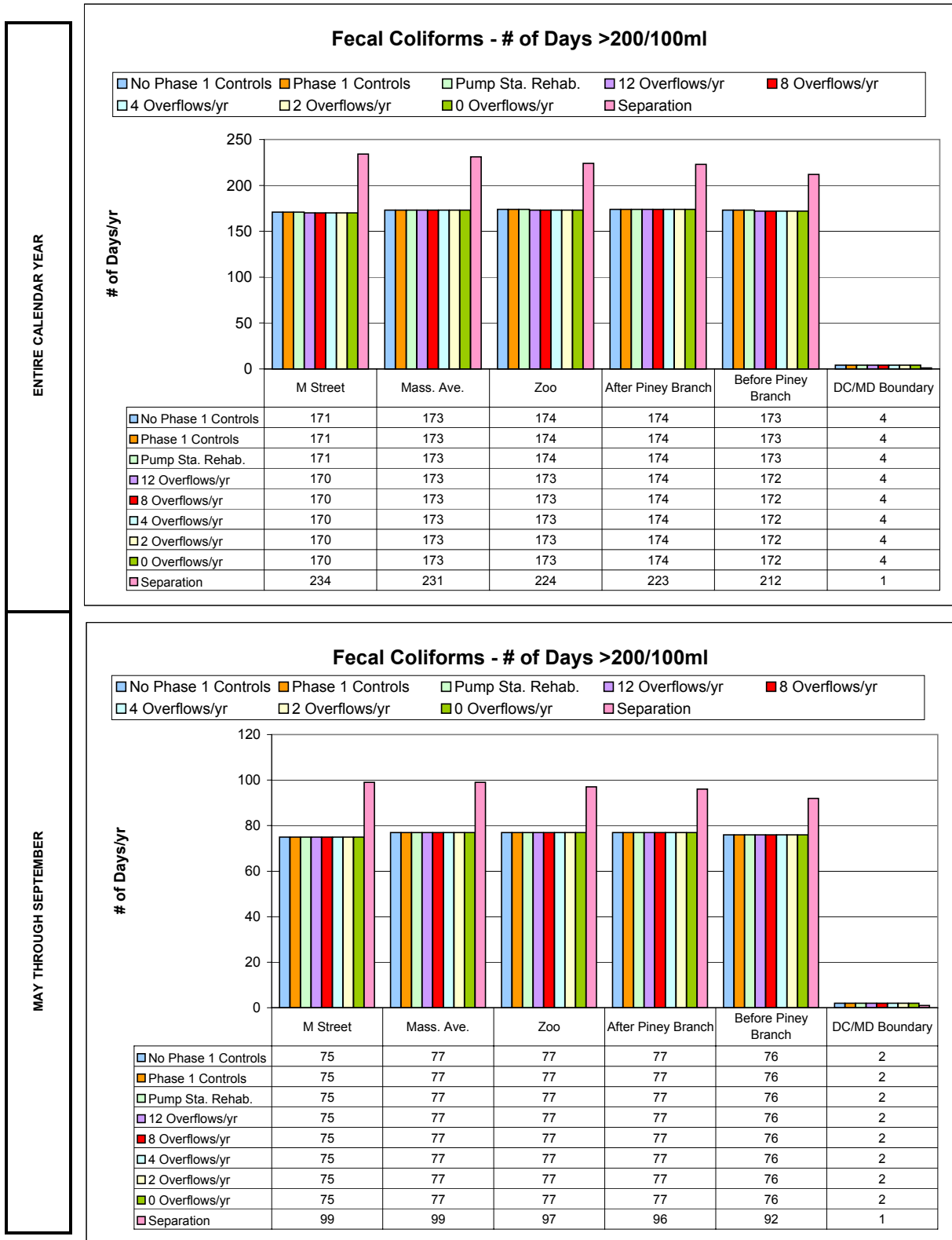
Figure D-15 Rock Creek: Effect of CSO Control on Fecal Coliform Concentrations (Upstream and Stormwater Load Reduction 1 )
