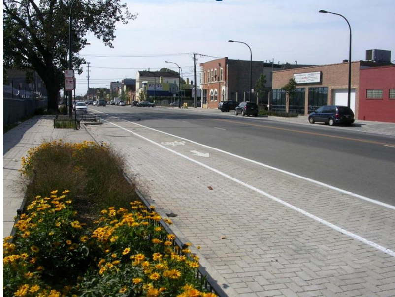
Alternate Permeable Parking Lane Materials
