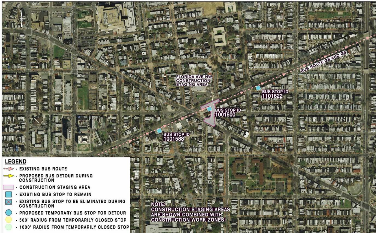
Figure 5-18 Study Area 3 - Existing Route G8, G9 and Bus Stop Locations along Eastbound Rhode Island Avenue (Florida Avenue Site)
