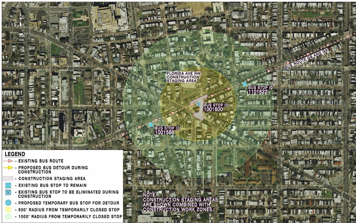
Figure 5-19: Study Area 3 – Existing Route G8, G9 and Proximity Map to Temporarily Closed Stops (Florida Avenue Site)
