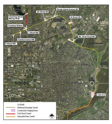
Figure 2-1. NEBT Alignment and Construction Sites
