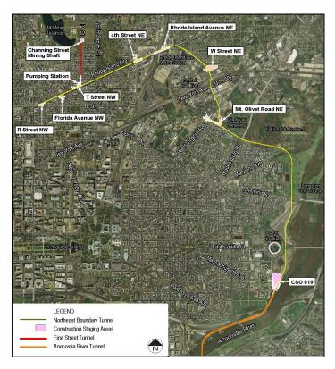
Figure 2-1. NEBT Alignment and Construction Sites
