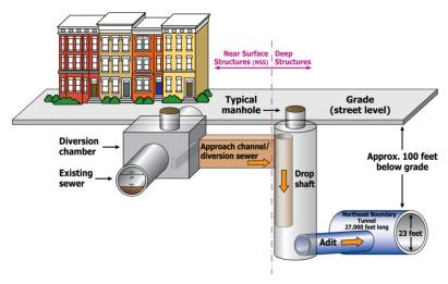
Figure 2-2: Graphic illustration of a typical diversion facility
