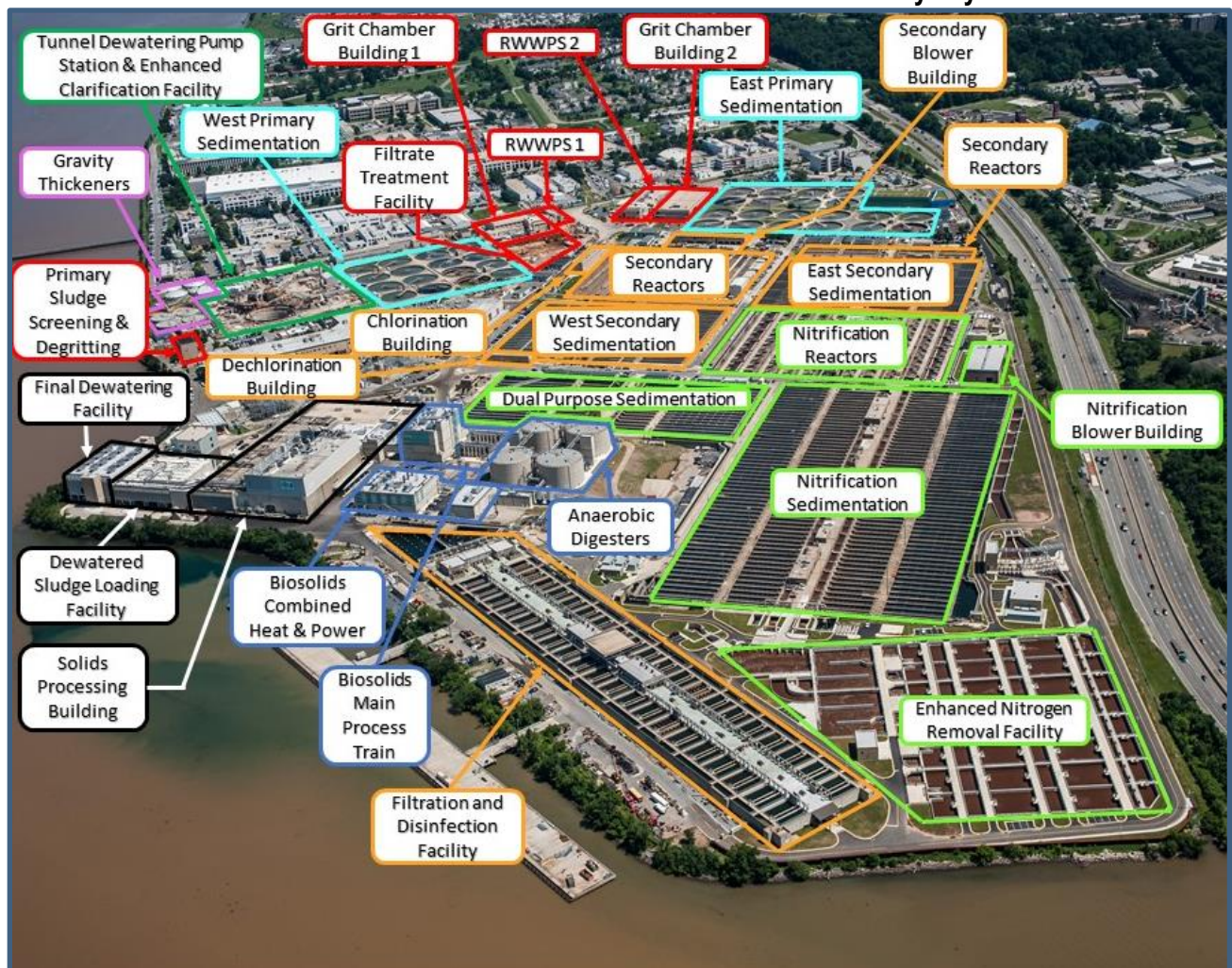
Exhibit 4-3: Blue Plains Wastewater Treatment Plant Facility Layout
