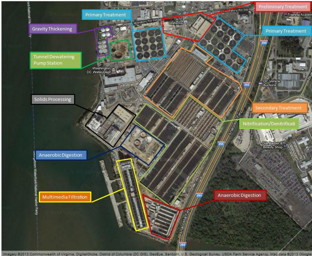
Exhibit 4.3-1: Blue Plains Wastewater Treatment Plant Site Plan (Satellite Image from Google Maps)
